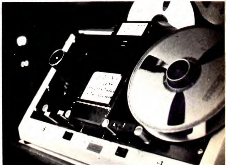
Early model of Recortec tape cleaner with razor blade attachment does better cleaning than Magnetek, says Reeves Broadcast which has both. But sign says do not use master tape.
